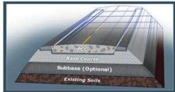
Typical Rigid Pavement
